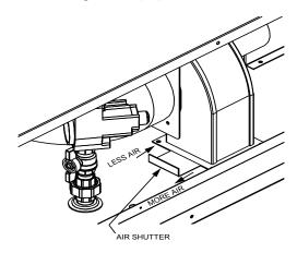
FIG. 56 Adjusting Air Shutter 399,999 - 750,000 Btu/hr Models
